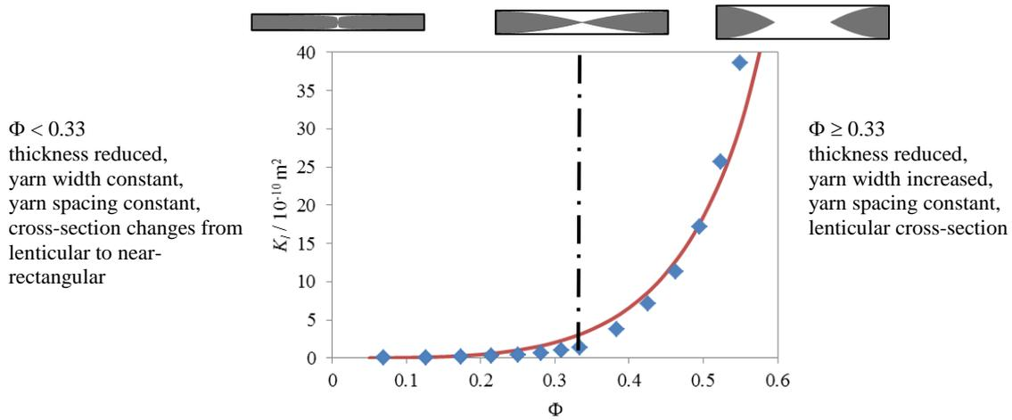
**Figure 2:** Example for permeability of a reinforcement layer,  $K_b$ , as a function of porosity,  $\Phi$ ; level of yarn compaction increases from right to left.
